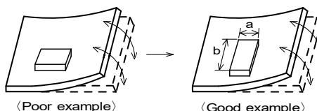
(2) Components location on PCB separation
