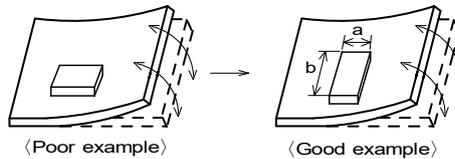
(2) Components location on PCB separation
