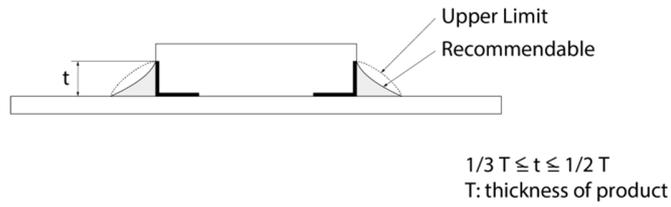
An increased solder volume increases mechanical stress on the product. Exceeding solder volume may cause the failure of mechanical or electrical performance.
