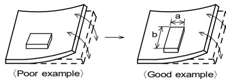
(2) Components location on PCB separation
