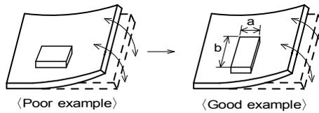
(2) Components location on PCB separation
