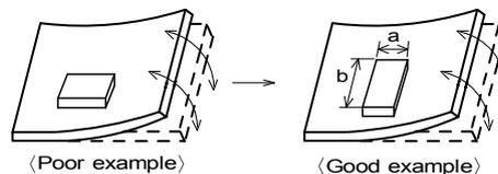
(2) Components location on PCB separation
