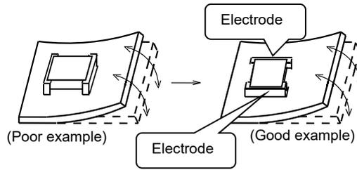
(2) Components location on PCB separation
