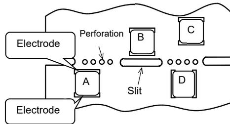
(3) Mounting components near screw holes
