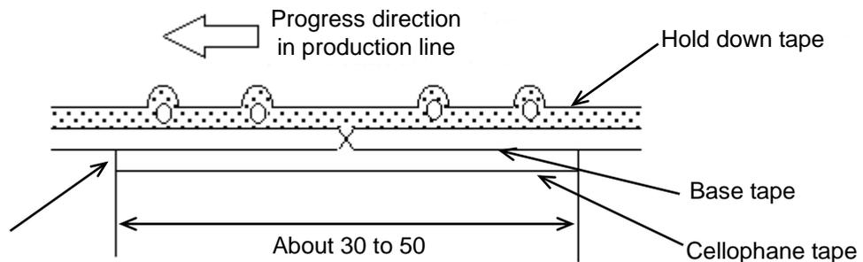
No lifting for the direction of progressing
