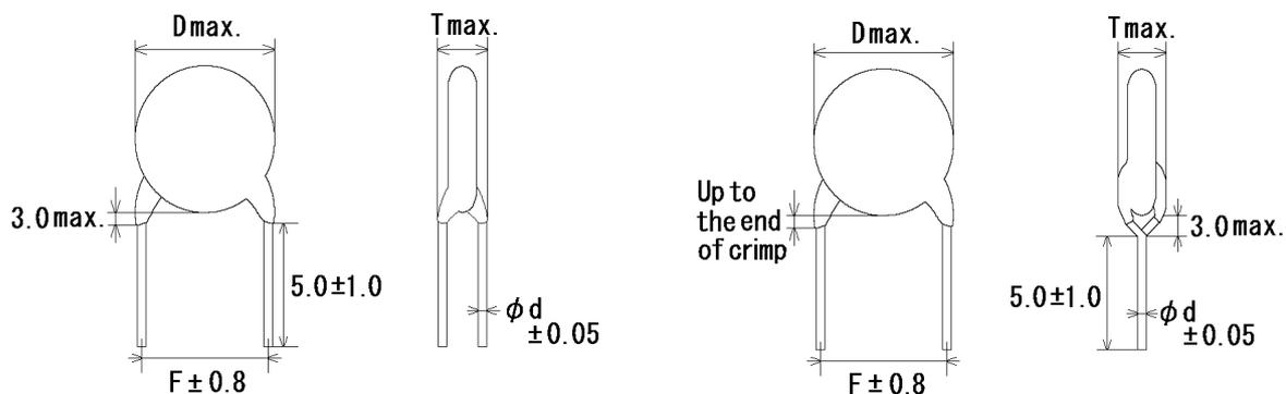
Note) The mark '\*' of lead code differ from lead spacing(F) and lead diameter(d).
