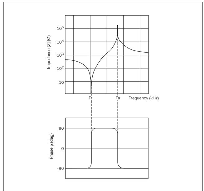
Fig. 2-2 Impedance and Phase Characteristics of CERALOCK
