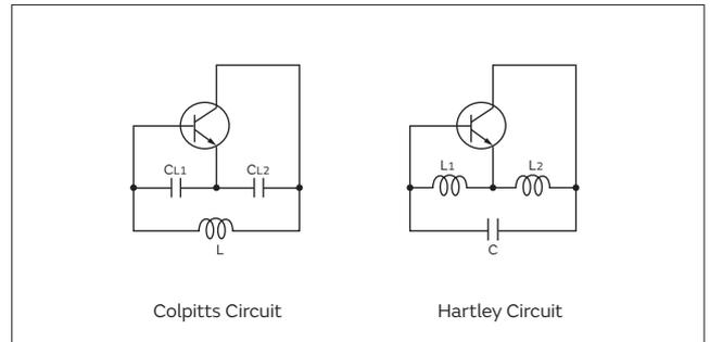
Fig. 2-6 Basic Configuration of LC Oscillation Circuit
