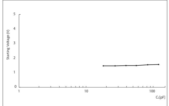
Fig. 5-6 Starting Voltage Characteristics against CL
