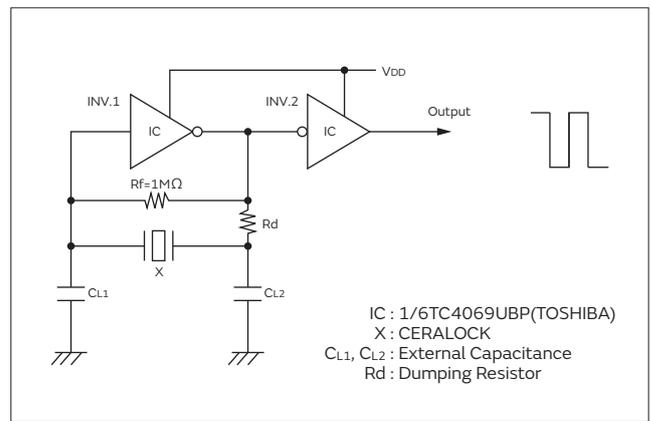
Fig. 4-1 Basic Oscillation Circuit with C-MOS Inverter
