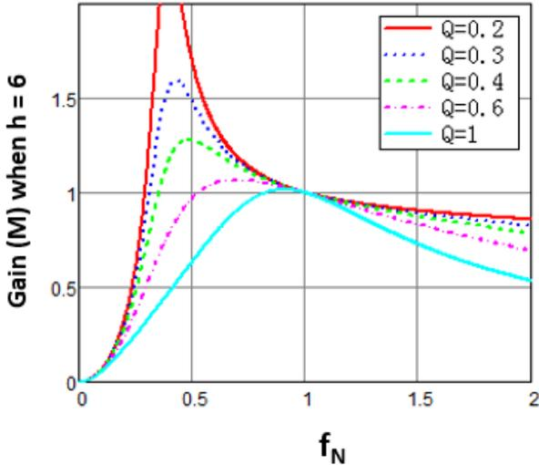
**Figure 22: Gain Curve vs. h and Q**
