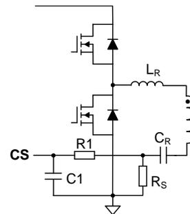
Figure 14: Current Sensing with a Current-Sense Resistor
