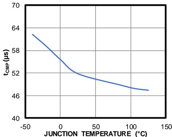
**BURST Threshold vs. Junction Temperature**
