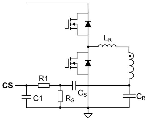
Figure 13: Current Sensing with a Lossless Network
