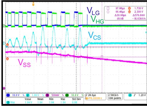
Figure 12: SCP Waveform
