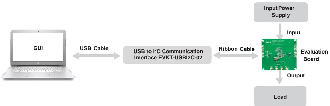
**Figure 1: EVKT-MP8833 Evaluation Kit Set-Up**
