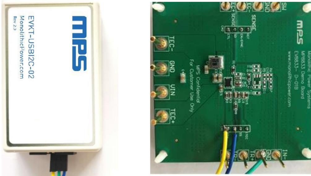
**Figure 6: EVB to MPS I<sup>2</sup>C Communication Interface Wire Connection**
