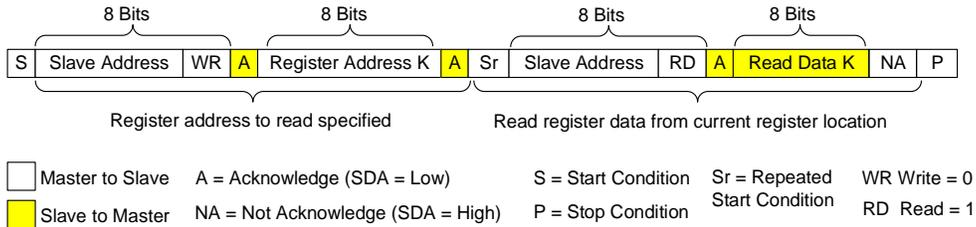
**Figure 15: I<sup>2</sup>C Read Example**
