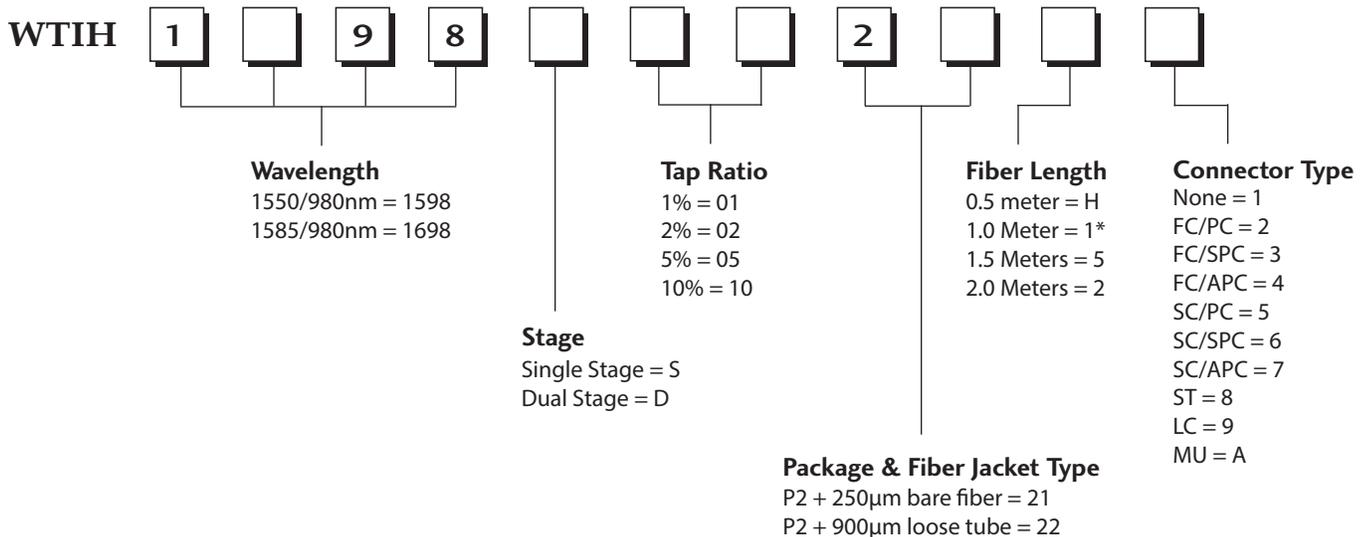
\* The tolerance of fiber length is +/-0.1m. 1 meter is standard.
