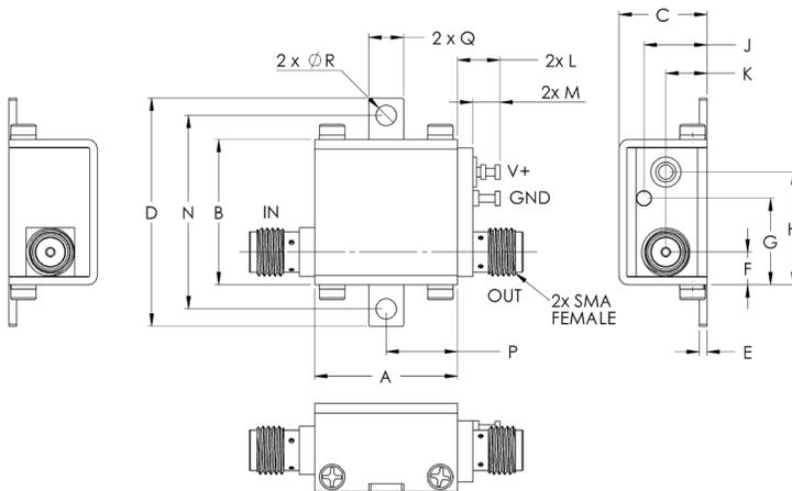
**!** NOTE: When soldering the DC connections, caution must be used to avoid overheating the DC terminal. See Application Note. [AN-40-010](#).
