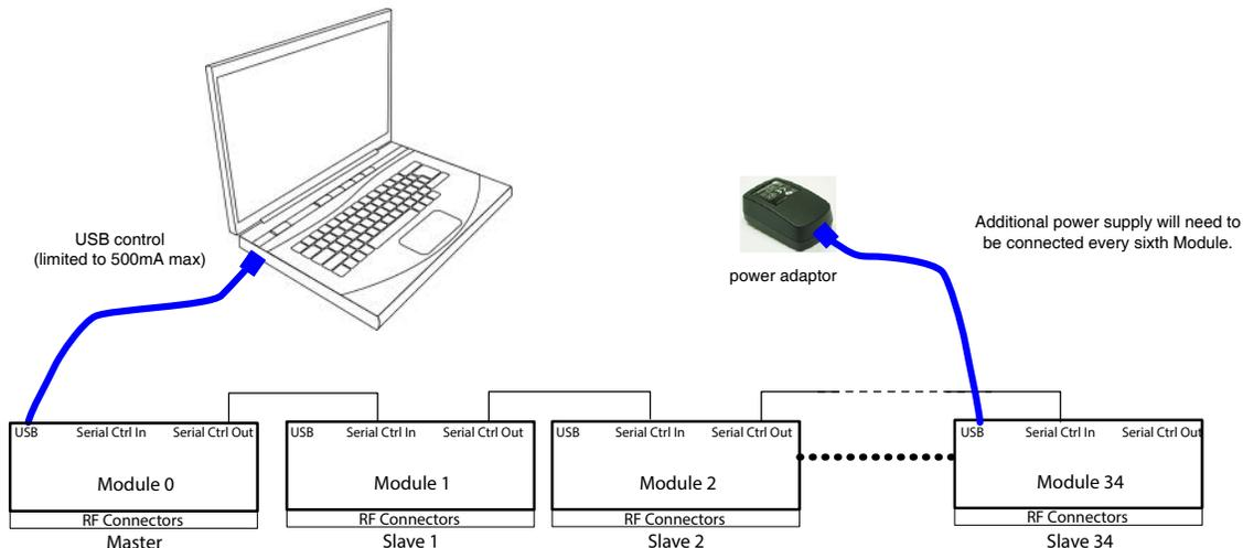
Connections between modules will be made using the serial in/out ports with the module connected to the PC as a master and all others as slave modules. All control will be through the master module (address zero) which is the only one communicating with the PC. Serial control out port of each module should be connected to the serial control in port of the next module. Power will be supplied from the PC via the master module up to a maximum of 500mA.
