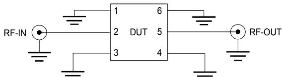
Fig 1. Block diagram of Test Circuit used for characterization, Test board TB-QAT-20C+
