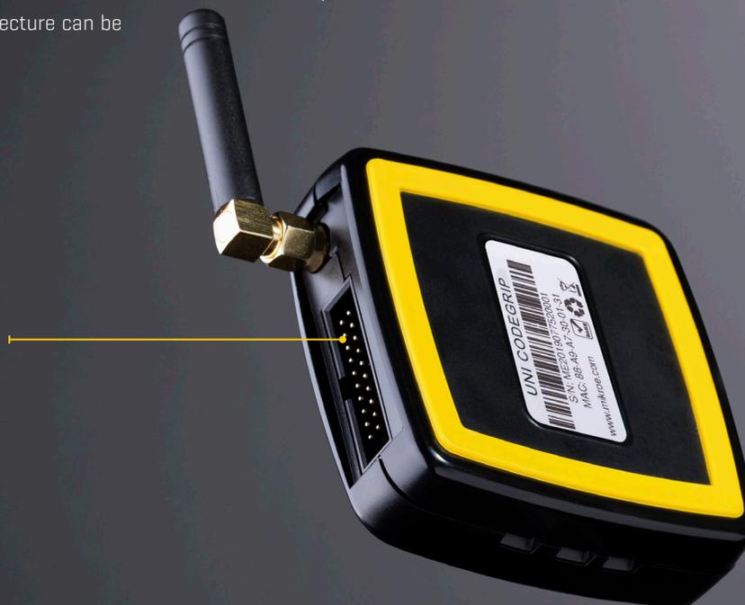
**NOTE** When the connected host board provides power to the CODEGRIP device, CODEGRIP input voltage must be in range 2.5V to 10V.
