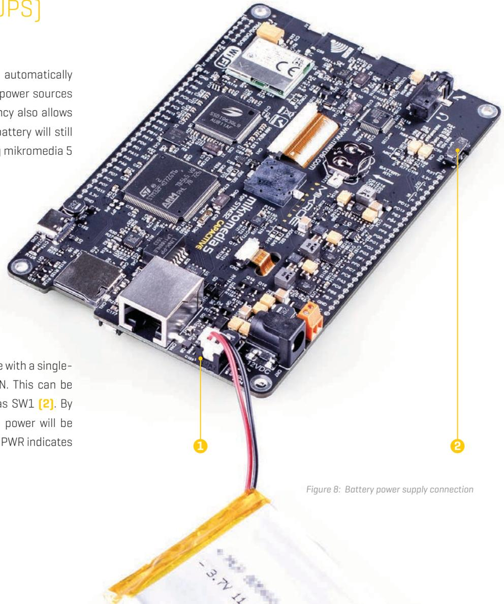
Figure 8: Battery power supply connection
