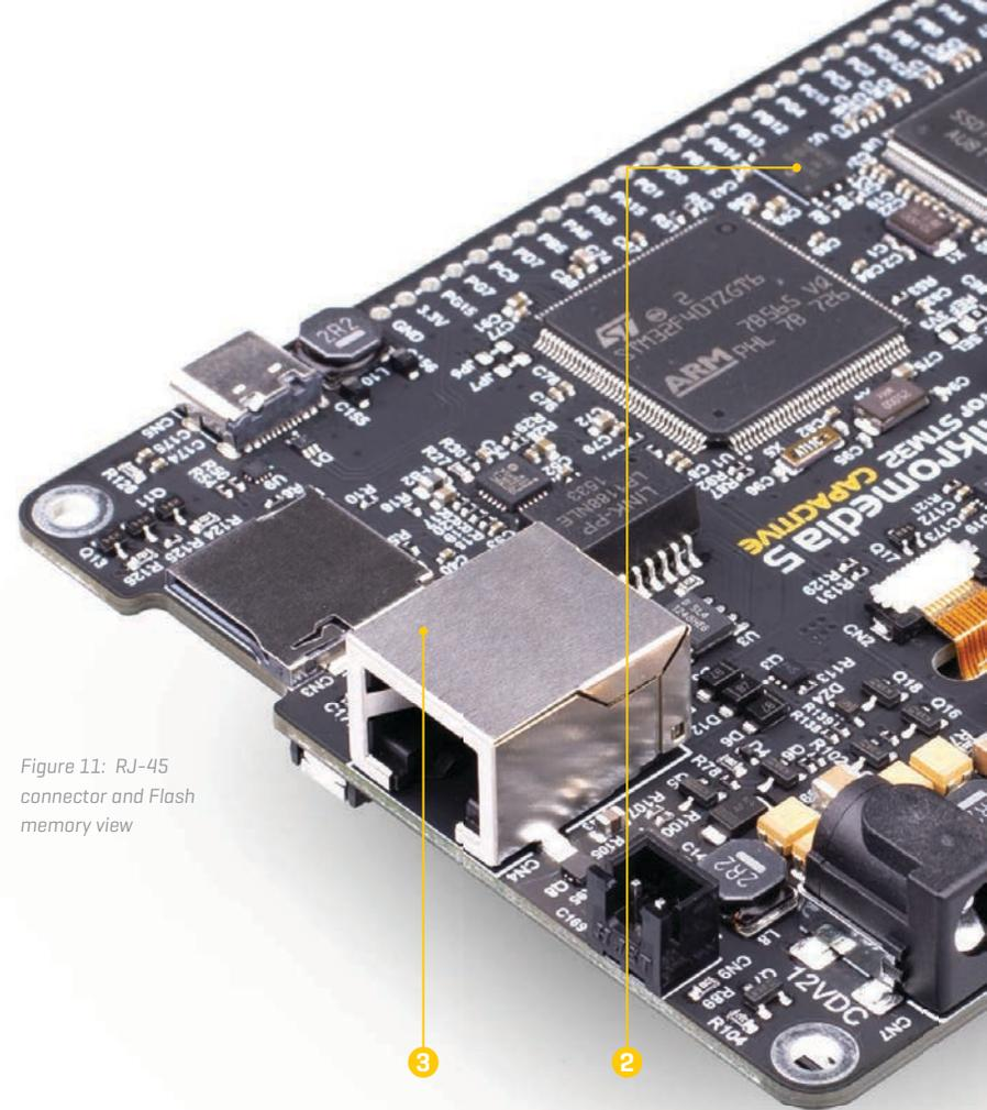
Figure 11: RJ-45 connector and Flash memory view
