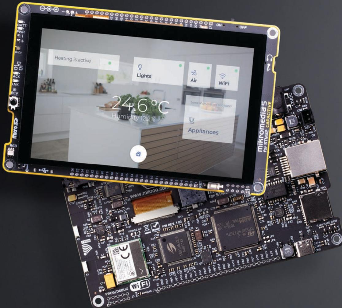
mikromedia 5 for STM32 CAPACITIVE is a compact development board designed as a complete solution for the rapid development of multimedia and GUI-centric applications. By featuring a 5" capacitive touch screen driven by the powerful graphics controller that can display the 24-bit color palette (16.7 million colors), along with a DSP-powered embedded sound CODEC IC, represents a perfect solution for any type of multimedia application.
