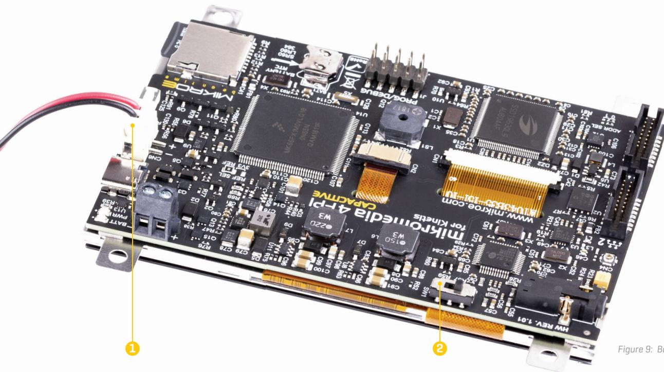
Figure 9: Battery power supply connection
