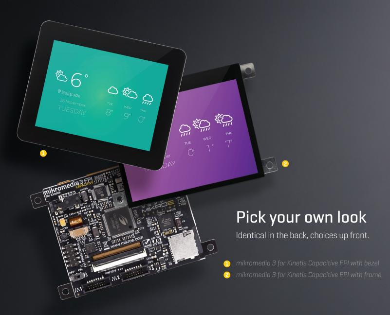
mikromedia 3 for Kinetis CAPACITIVE FPI is a compact development board designed as a complete solution for the rapid development of multimedia and GUI-centric applications. By featuring a 3.5" capacitive touch screen driven by the powerful graphics controller that can display the 24-bit color palette [16.7 million colors], along with a DSP-powered embedded sound CODEC IC, represents a perfect solution for any type of multimedia application.
