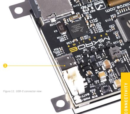
power over the USB-C connector **(1)** for the attached DEVICE. The USB PSW pin is driven by the host MCU, allowing the software to control the USB mode.
