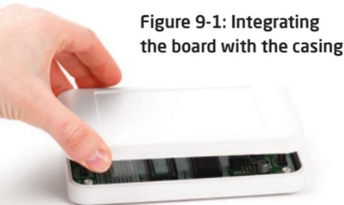
**Figure 9-1: Integrating the board with the casing**
