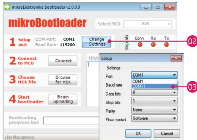
Figure 5-2: UART mikroBootloader
