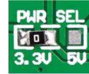
On-board **PWR SEL** zero-ohm resistor (SMD jumper) is used to determine whether 5V or 3.3V power supply is used. This resistor is provided in 3.3V position by default. In order to use SHT1x click with 5V development system, it is necessary to resolder this jumper to 5V position.
