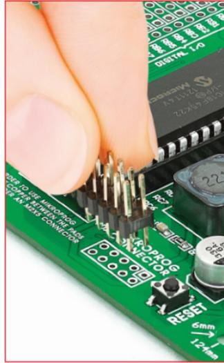
Figure 3-3: placing 2x5 male header
