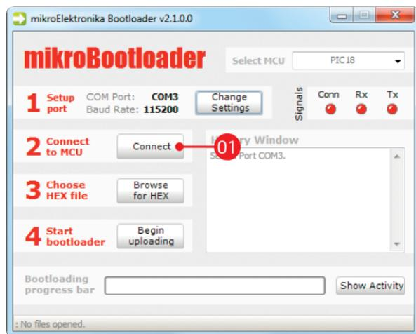
Figure 2-4: Connecting with mikroBootloader
