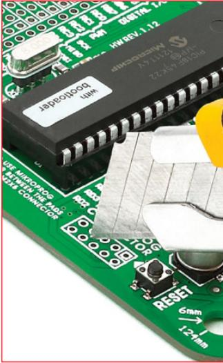
Figure 3-2: cutting copper between pads
