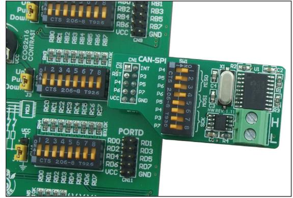
Figure 2: CAN-SPI board connected to a development system
