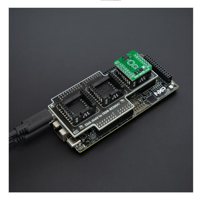
When the USB type C is connected to the Click Shield and the other USB is connected to the FRDM-MCXN947 board, the PWR diode will glow Cyan, and at this setup, the mikroBUS $^{\text{m}}$  sockets are powered from the Click Shield.
