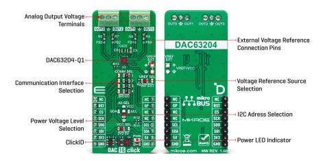
The DAC63204-Q1 supports flexible configuration of its output channels (OUT0-OUT3). For voltage outputs, it provides a 1LSB differential non-linearity (DNL) and allows for adjustable gains, with options of 1x, 1.5x, 2x, 3x, and 4x. For current outputs, it offers a range of  $\pm 25\mu$ A to  $\pm 250\mu$ A, with 1LSB integral non-linearity (INL) and DNL (8-bit), making it suitable for precision applications requiring fine control over current delivery.
