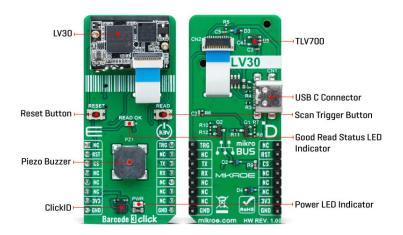
The LV30 is equipped with a red LED (wavelength:  $625\pm10$ nm) for additional lighting, allowing for barcode scanning even in complete darkness, with the option to turn the illumination ON or OFF. It also includes a laser aimer to help users accurately position the barcode within the scanning area, enhancing efficiency. The aiming pattern can be toggled ON or OFF, with the recommendation to keep it on during scanning for better accuracy.
