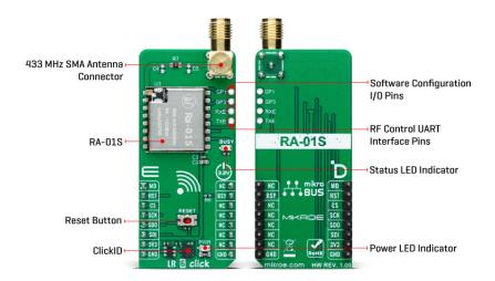
Compared to traditional modulation technologies, LoRa™ offers significant advantages regarding anti-blocking and signal selection, addressing distance, interference, and power efficiency challenges. LR 6 Click is well-suited for various applications such as automatic meter reading, home and building automation, security systems, and remote irrigation systems, where long-distance communication and reliability are critical.
