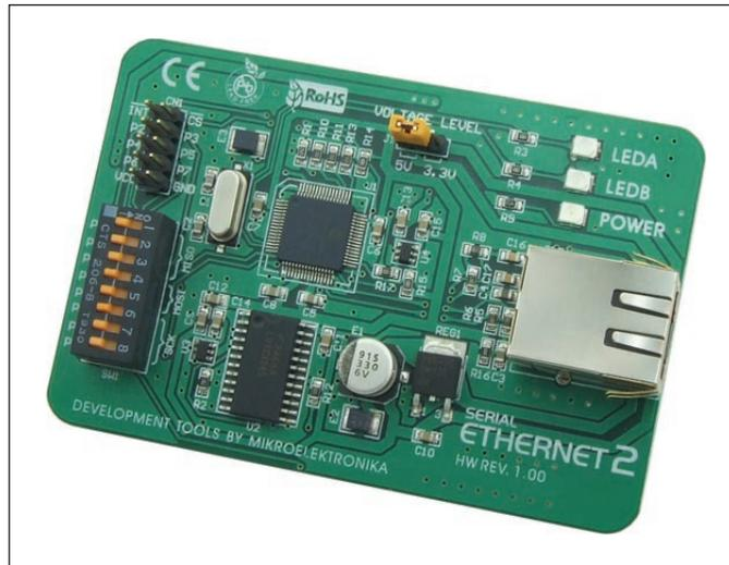
Figure 1: Serial Ethernet2 additional board
