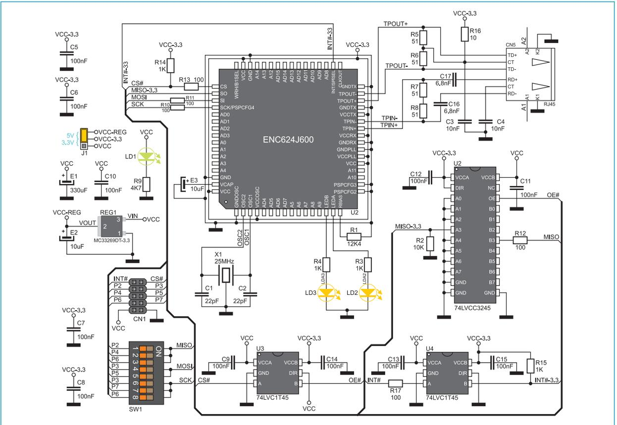
Figure 3: Serial Ethernet2 board connection schematic
