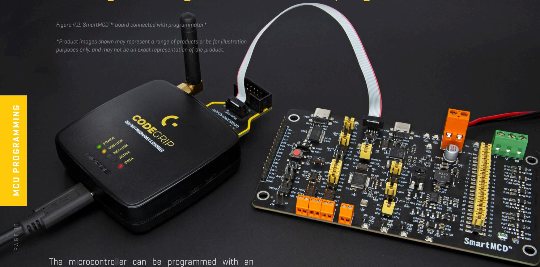
The microcontroller can be programmed with an external programmer and supported software. The external programmer is connected to the development board via a 2x5 PROG/DBG connector soldered on the J4 connector pads.
