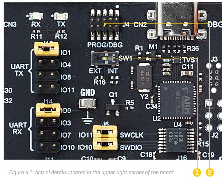
Figure 4.1: Actual details located in the upper right corner of the board.
