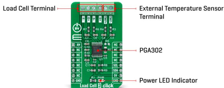
The PGA302 contains two separated analog-front end (AFE) chains with their gain amplifiers for resistive bridge and temperature sensing inputs. The resistive bridge input AFE chain consists of a programmable gain with eight steps from 1.33V/V to 200V/V. For the temperature-sensing input AFE chain, the PGA302 provides a current source that can source up to 1mA for the optional external temperature sensing available on the on-board terminal labeled with TMP+ and TMP-.
