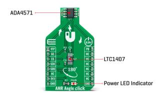
The ADA4571 contains two Wheatstone bridges, at a relative angle of 45° to one another. A rotating magnetic field in the x-y sensor plane delivers two sinusoidal output signals with the double frequency of the angle between sensor and magnetic field direction. Within a homogeneous field in the x-y plane, the output signals are independent of the physical placement in the z-direction (air gap).
