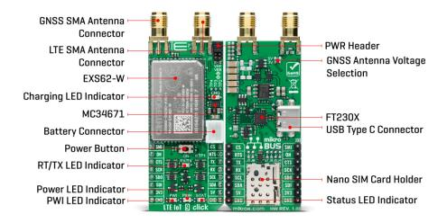
This Click board  $^{\text{\tiny TM}}$  is equipped with a USB type C connector. It allows the module to be powered and configured by a personal computer (PC) using  $\underline{\mathsf{FT230X}}$ , a compact USB to a serial UART interface device designed to operate efficiently with USB host controllers. It uses as little bandwidth as possible when compared to the total USB bandwidth available.
