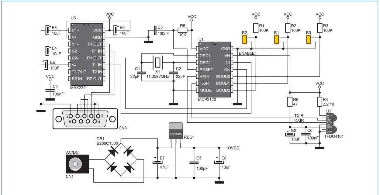
Figure 3: IrDA to PC additional board connection schematic
