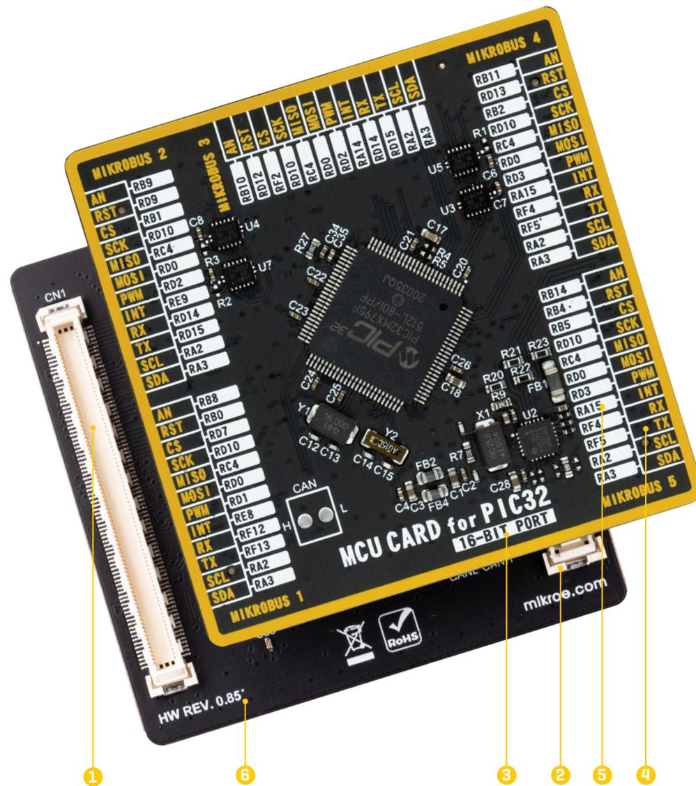
Figure 7: MCU card back and front view
