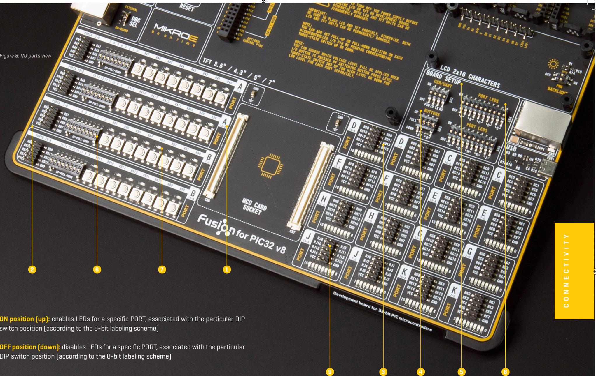
**ON position [up]:** enables LEDs for a specific PORT, associated with the particular DIP switch position [according to the 8-bit labeling scheme]
