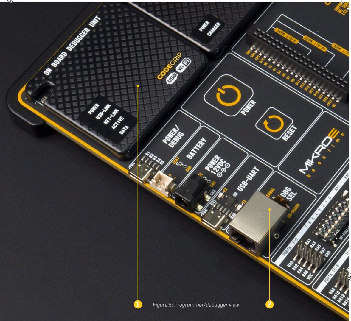
Figure 5: Programmer/debugger view
