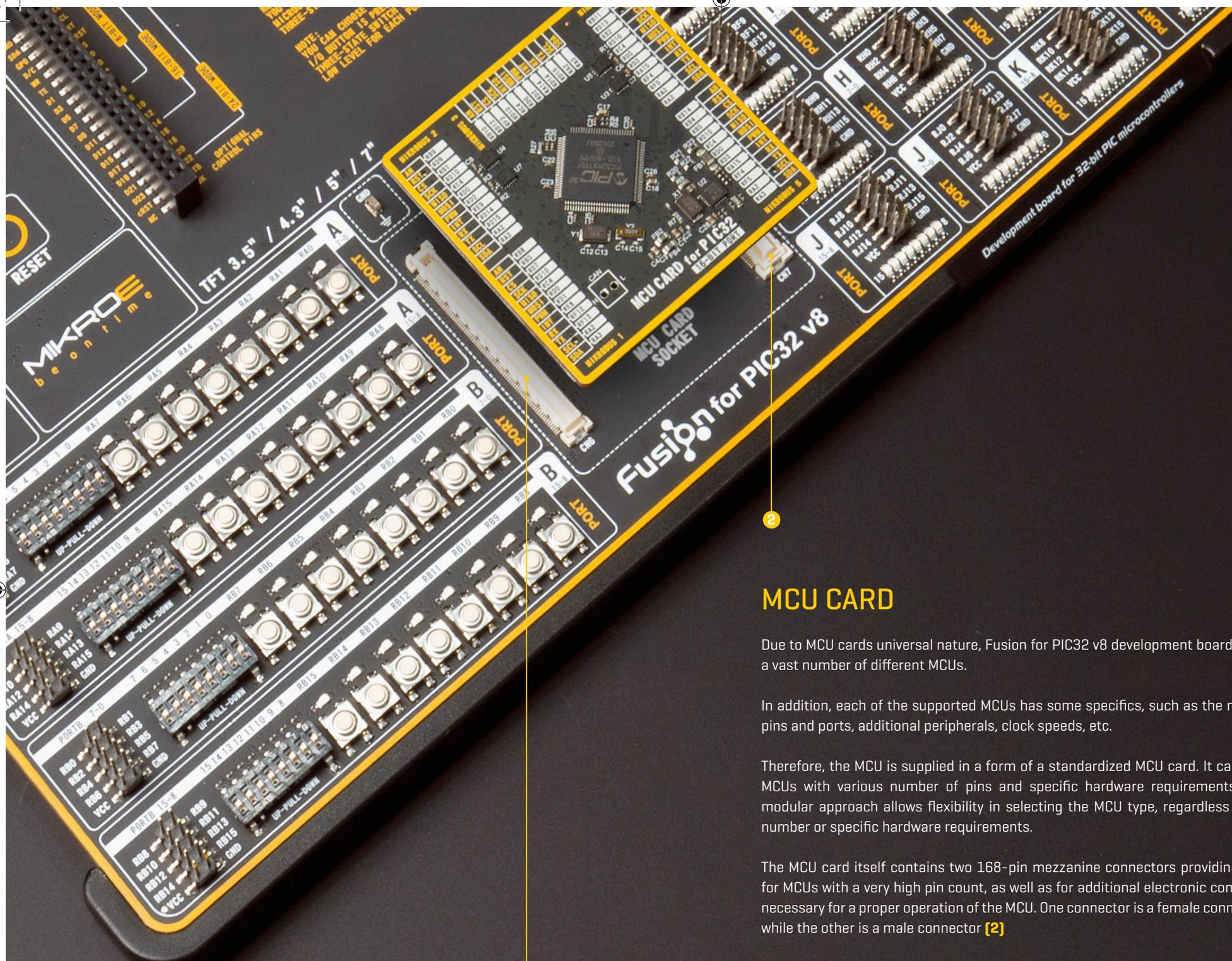
Figure 6: Main board with MCU card socket view
