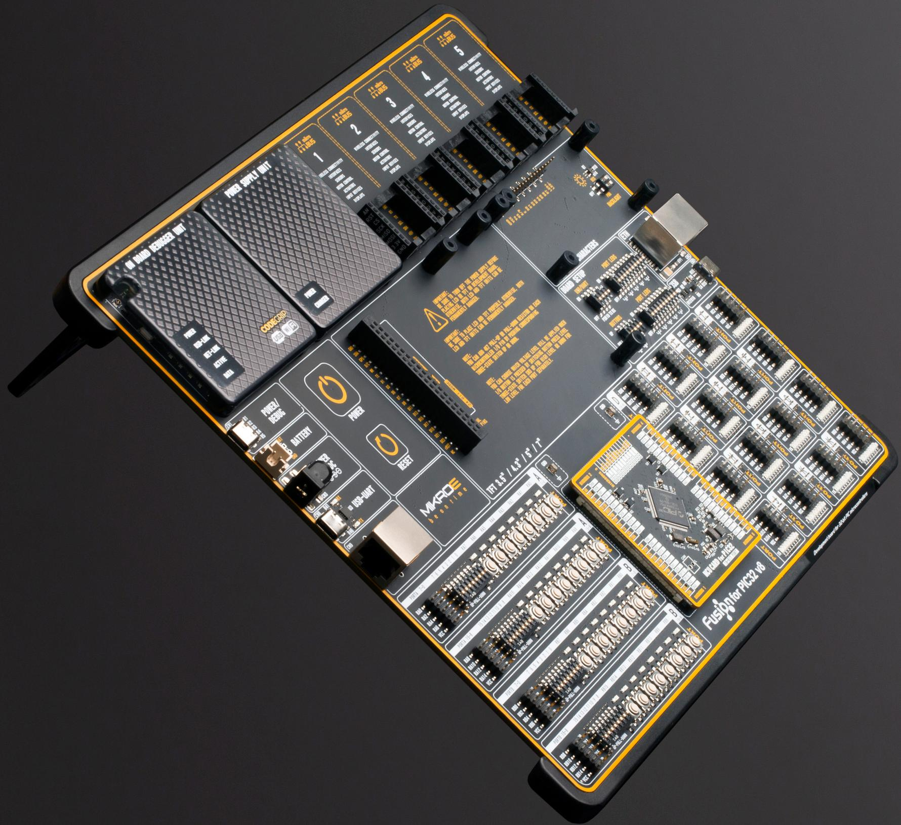
**Fusion for PIC32 v8** is a development board designed for rapid development of embedded applications. Redesigned from the ground up, it offers broad **set of standard**, as well as several **unique features** never seen before in the world of embedded electronics: **programming and debugging over WiFi network**, support for a large number of **Microchip's PIC32** microcontrollers regardless of their pin number and more.
