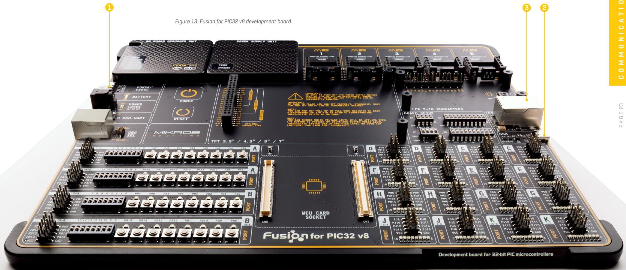
Figure 13: Fusion for PIC32 v8 development board
