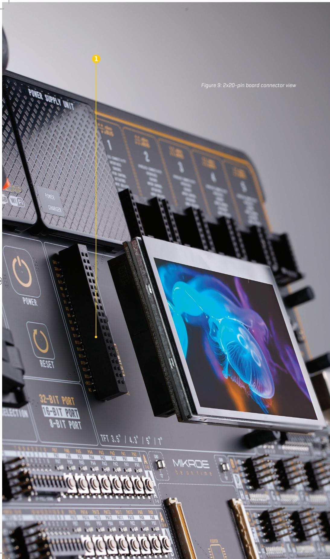
Figure 9: 2x20-pin board connector view
