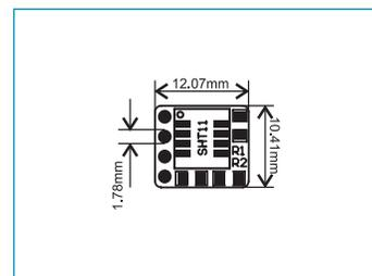
Figure 3: Dimensions of the board
