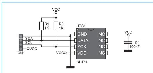
Figure 2: SHT1X PROTO board connection schematic
