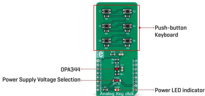
By pressing a button, the respective connection point becomes redirected to the input of the [OPA344](#), a low-power operational amplifier from [Texas Instruments](#), which is configured to work with the unity gain, forming a buffer for the input of the microcontroller (MCU). This prevents changes of the impedance at the MCU input pin, as well as a limited amount of ESD protection.
