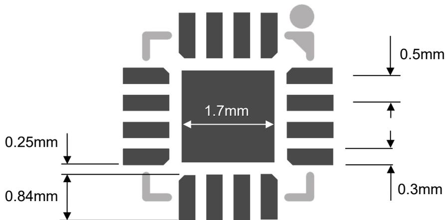
Figure 7.2 IQS266 Recommended PCB footprint
