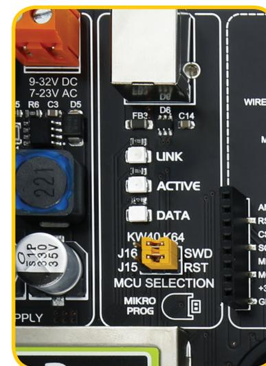
Figure 10: Programmer LEDs
