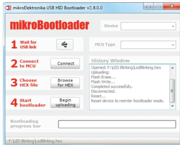
Figure 1-7: mikroBootloader ready for next job
