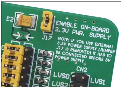
**Figure 7:** Jumper J17 placed on the board
