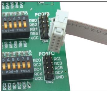
Figure 2: Plugging IDC10 connector into a development system
