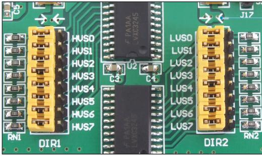
**Figure 4:** Jumpers DIR1 and DIR2 in the position for 5V to 3.3V voltage level adjustment
