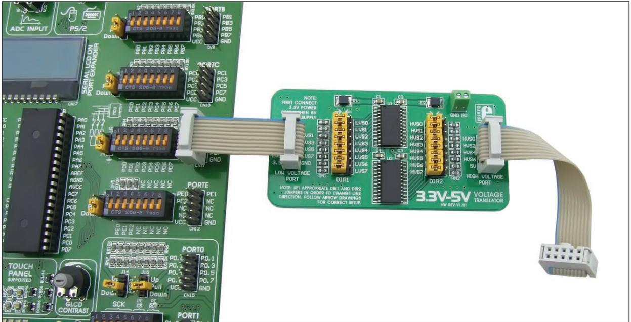
Figure 4: 3.3V-5V VOLTAGE TRANSLATOR board connected to a development system
