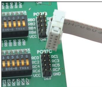
Figure 2: Connecting IDC10 connector to a development system
