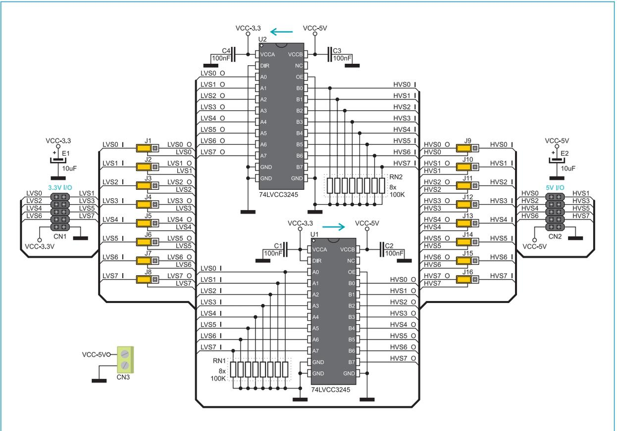
Figure 6: 3.3V-5V VOLTAGE TRANSLATOR board connection schematic
