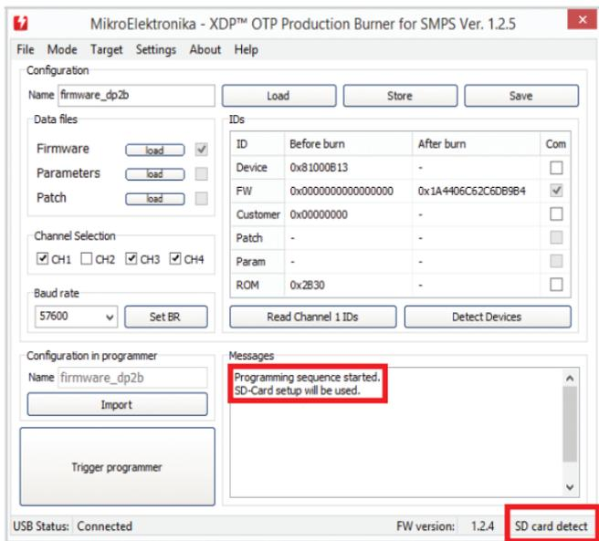
MicroSD card must be formatted with FAT32 file system. To load the configuration setup to an microSD card, simply copy the configuration [“.cfg”] file to previously formatted card — just a single file, without additional files or folders. Single configuration file must be located in the root folder of the microSD card.
