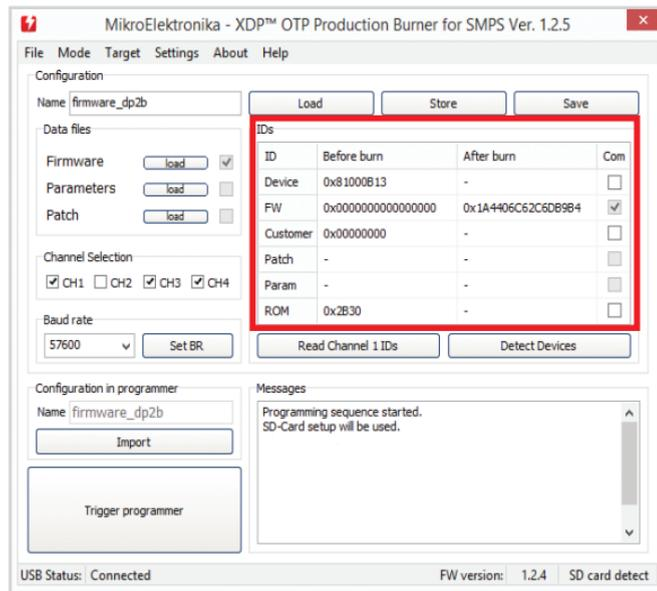
Note the **XXXX** parameter value in the Before burn column [1 on left image]. This indicates that the config file includes a full set parameter update, making the Before burn parameter value irrelevant. The Before burn parameter ID
