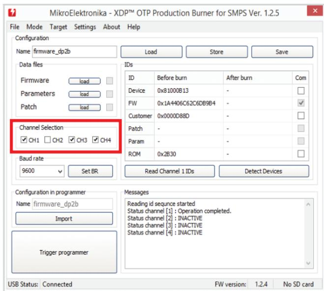
The user can specify which target devices are to be programmed, by selecting active channels. This is done by ticking corresponding CH1-CH4 checkboxes in the Channel Selection section. The XDP™ OTP Burner will program only target devices connected to the selected channels. The
