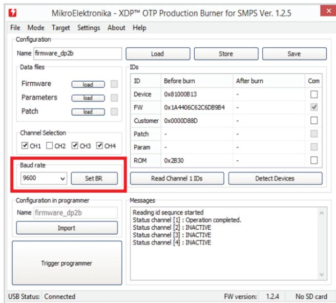
The XDP™ OTP Burner communicates with SMPS devices through a specialized one-wire UART interface. The
