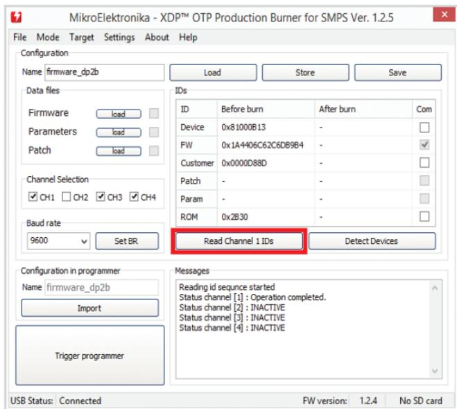
that are required to match will have corresponding check box ticked in the upper right pane of the table interface. The table will also list “After burn” IDs for reference.
