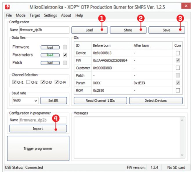
In order to properly configure the XDP™ OTP Burner, the selected configuration setup must be stored to XDP™ OTP Burner device by clicking the Store [2] button. Only after a successful execution of this operation, the XDP™ OTP
