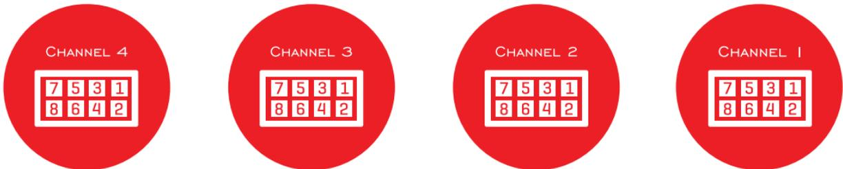
Each channel has an 8 pin connector [IDC8]. The function of each pin is identical on each channel — except for pin #6. The sixth pin in each channel indicates an “overall” event, that is, a signal that applies not just to that particular channel, but to all channels together. The purpose of these “overall” pins is to enable users to connect a custom external circuit to monitor the programming process. This is an optional feature, not necessary for ordinary use.
