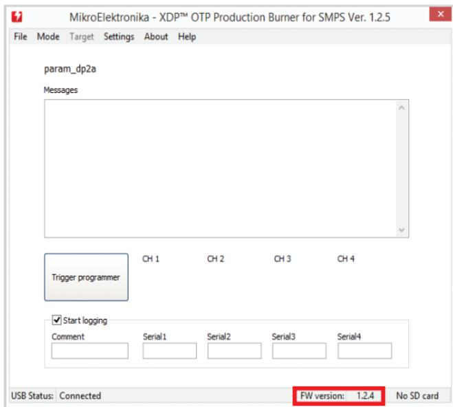
The XDP™ OTP Burner comes pre-programmed with MikroElektronika's USB-HID Bootloader. This feature enables firmware updates over the USB. A Windows application called mikroBootloader is required to complete the process. For instructions on how to change the firmware using the mikroBootloader app, refer to [docs.mikroe.com/MikroBootloader](https://docs.mikroe.com/MikroBootloader)
