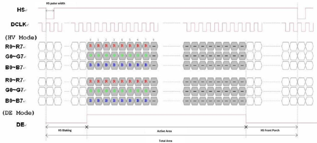
Figure 10. Vertical input timing diagram
