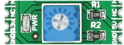
To calibrate Alcohol click™ for optimum performance, use the on-board potentiometer to adjust the Load Resistance of the sensor circuit.
