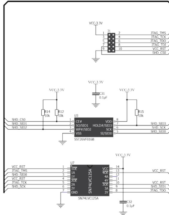
Figure 4-13: mikroProg™ connection schematic
