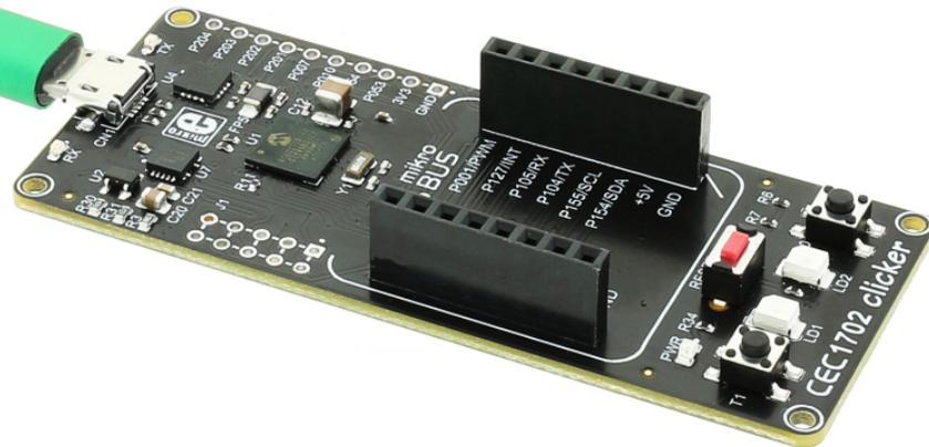
When the board is powered up the power indication LED will be automatically turned on. The USB connection can provide up to 500mA of current which is more than enough for the operation of all on-board and additional modules.
