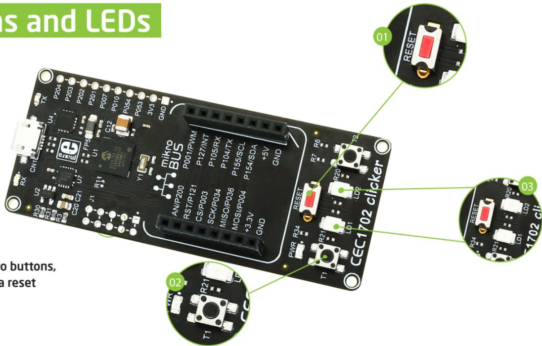
Figure 5-1: Two buttons, two LEDs and a reset button
