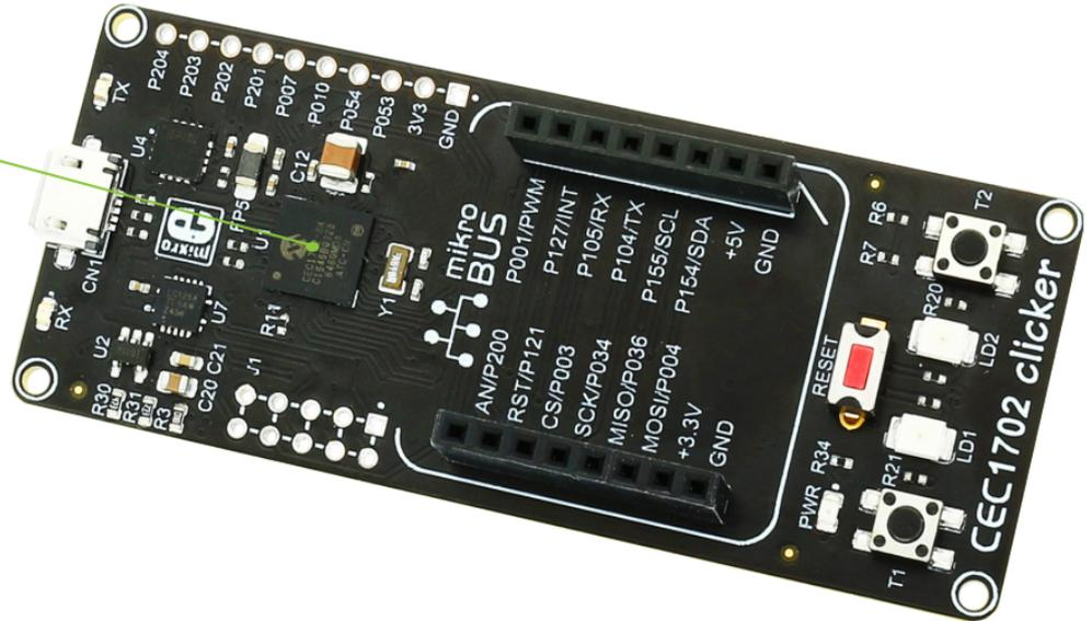
The microcontroller can be programmed using external mikroProg™ for CEC1702 programmer.
