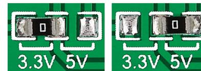
Button G click has a PWR SEL jumper [zero ohm resistor] that lets you switch between 3.3V and 5V power supplies.
