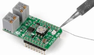
Turn the board upward again. Make sure to align the headers so that they are perpendicular to the board, then solder the pins carefully.
