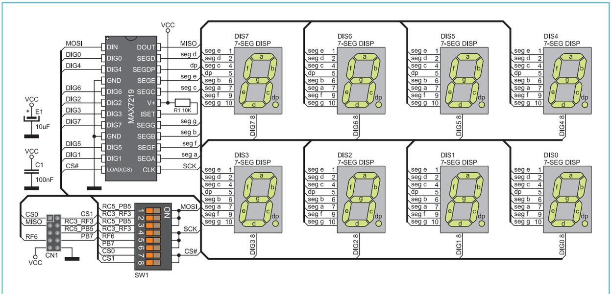
Figure 2: Serial 7-Seg Display 2 additional board connection schematic
