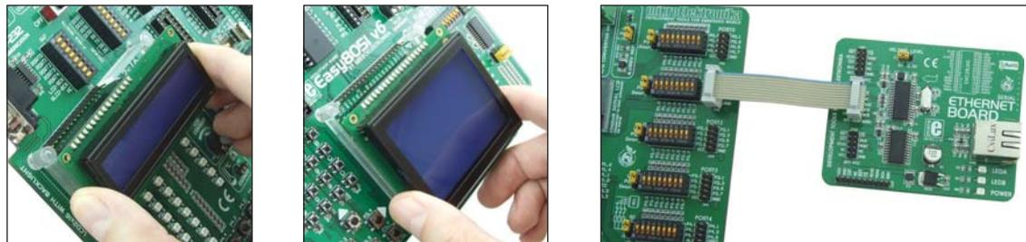
Figure 1-3: Placing additional modules on the board
