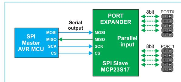
Figure 18-3: SPI communication block diagram
