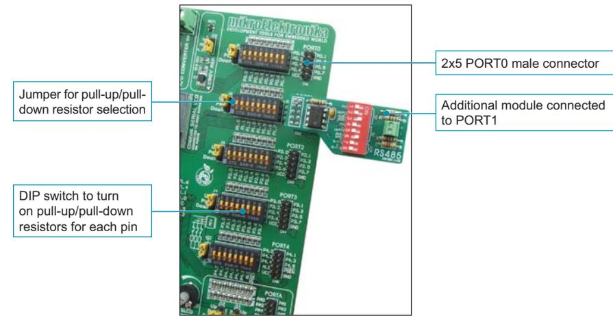
Figure 17-1: I/O ports
