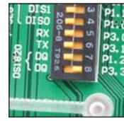
**Figure 8-4:** Switch 8 on the DIP switch SW8 is in the ON position, DS1820 is connected to the P3.3 pin
