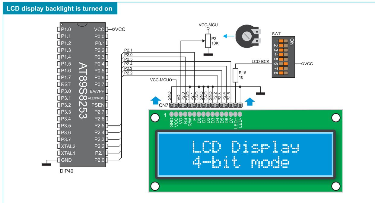
Figure 14-3: Alphanumeric 2x16 LCD display connection schematic
