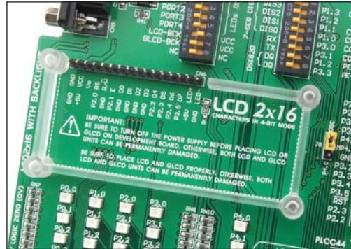
Figure 14-1: Alphanumeric 2x16 LCD display connector
