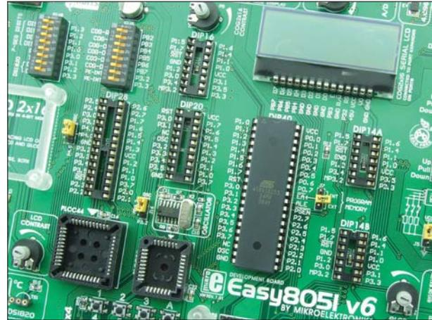
Figure 2-1: Microcontroller sockets
