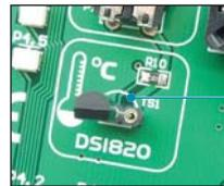
**Figure 8-2:** DS1820 is plugged into the connector
