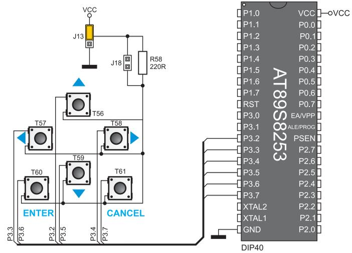
Figure 11-2: MENU keypad and microcontroller connection schematic
