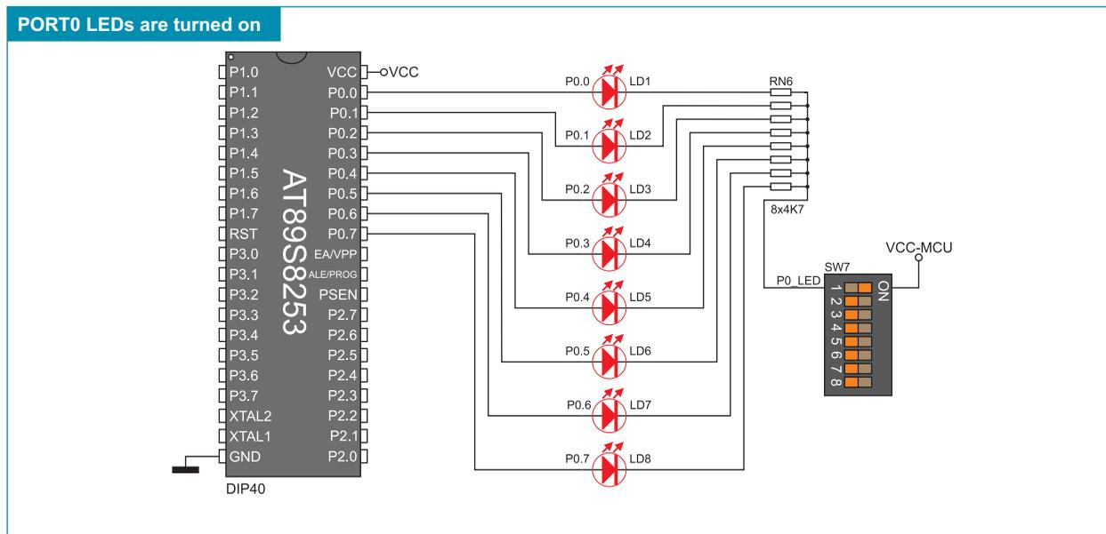
Figure 9-2: LED diode and port PORT0 connection schematic
