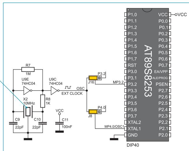
Figure 4-2: Oscillator schematic
