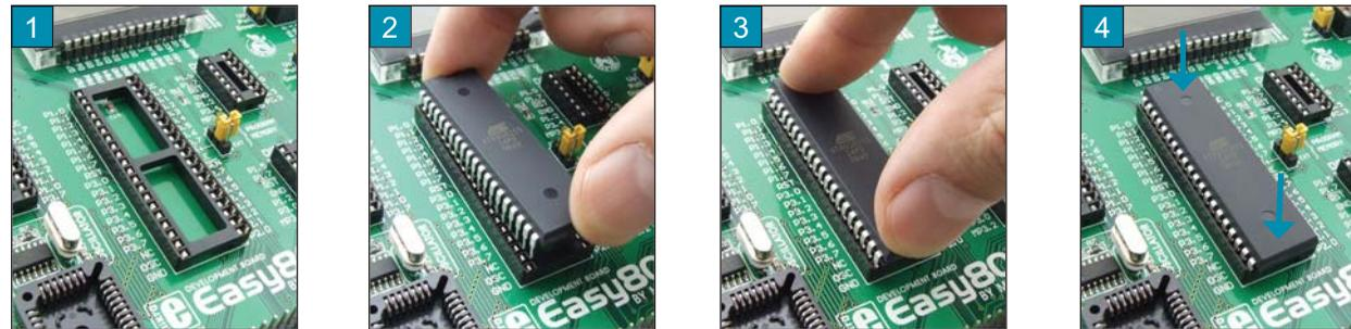
Figure 2-2: Plugging a microcontroller into appropriate socket
