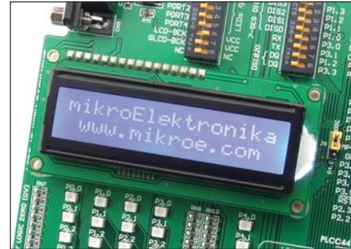
Figure 14-2: Alphanumeric 2x16 LCD display
