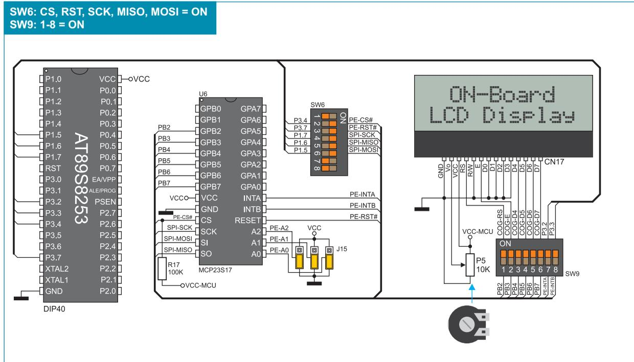
Figure 13-2: On-board LCD display connection schematic
