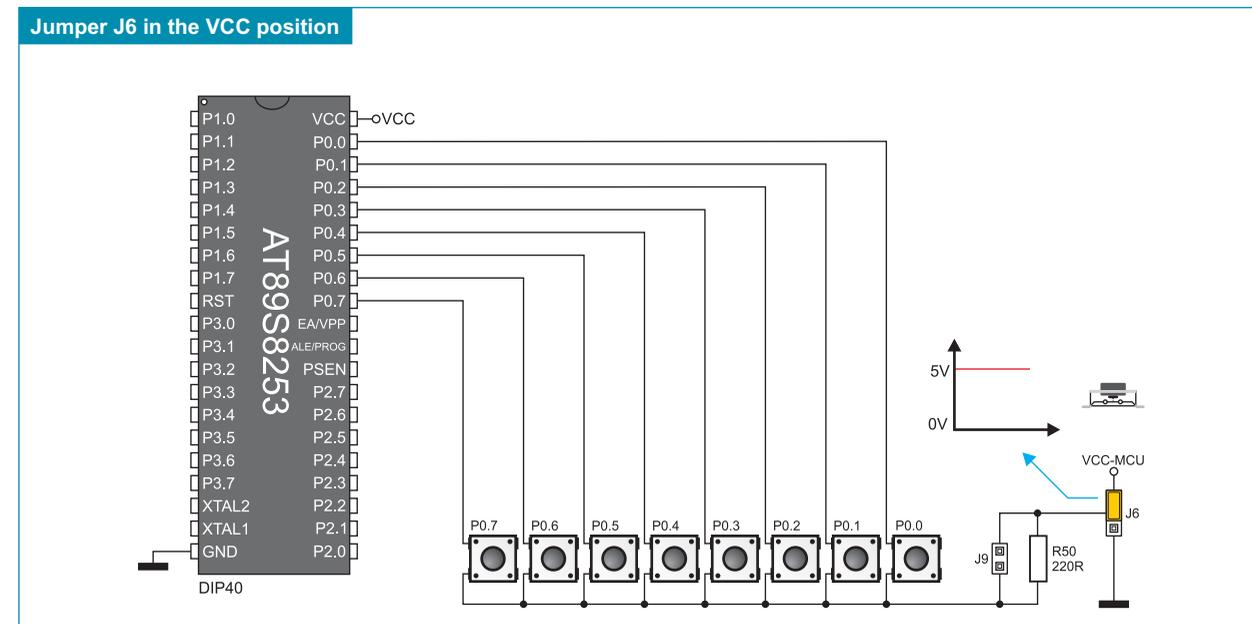
Figure 10-2: Push buttons and port PORT0 connection schematic
