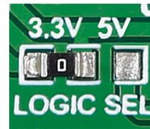
LOGIC SEL is used to determine whether 5V or 3.3V logic level is used on the interrupt pins.
