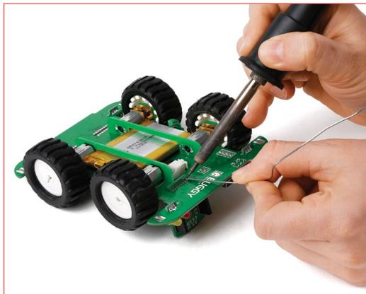
**STEP 8 -** Solder mikroBUS™ socket plates
