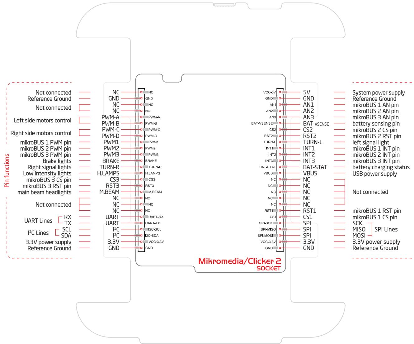
The Buggy carries a standard clicker 2/mikromedia pinout with a pair of 1x26 connection pads. However, to make the Buggy easier to program, some of the pins have descriptive labels that point out their functions in relations to the motors, lights and so on.
