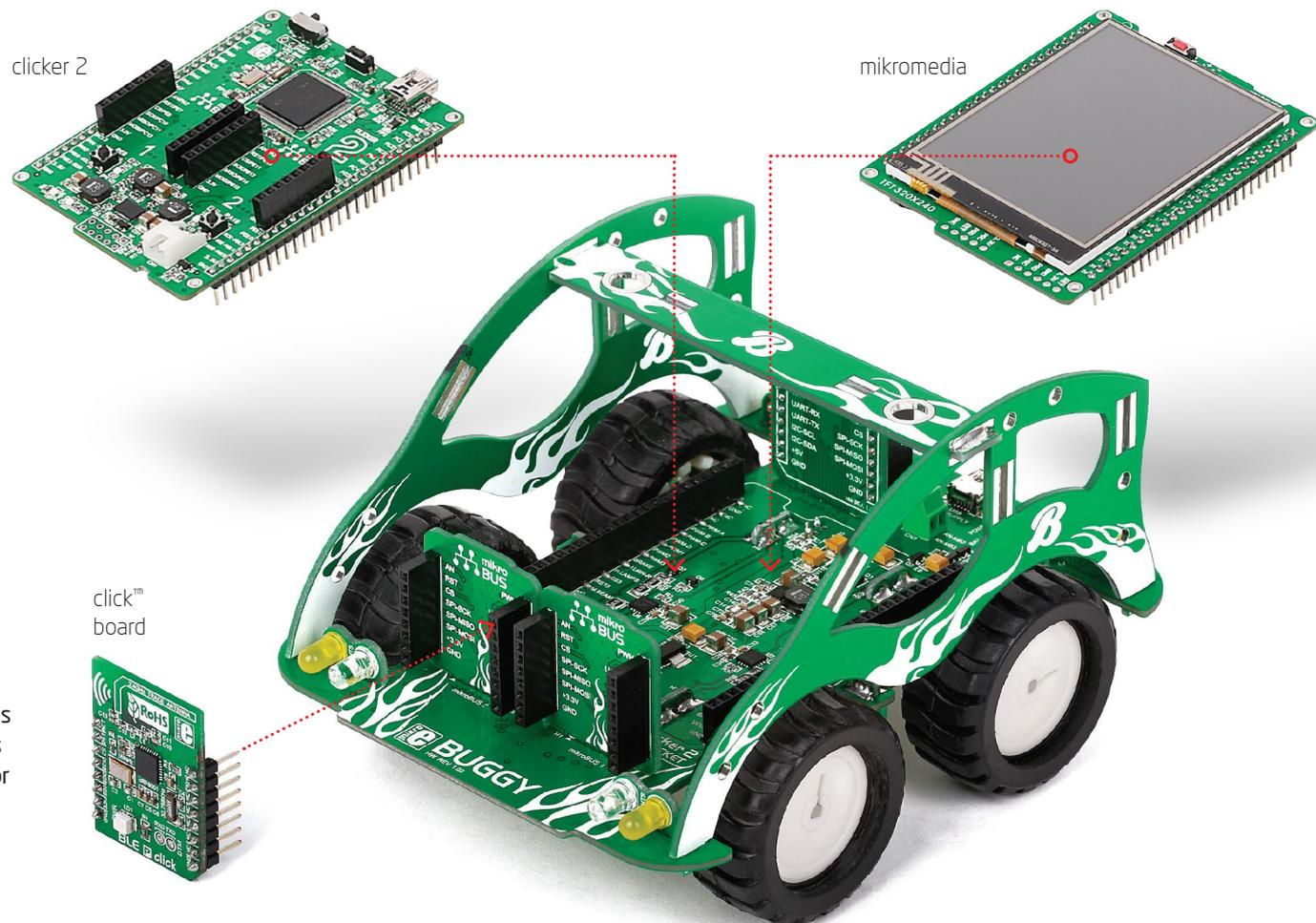
If you want to remotely control your Buggy, you'll also need a communications click™ board with a wireless transceiver module (Wi-Fi or Bluetooth work well).
