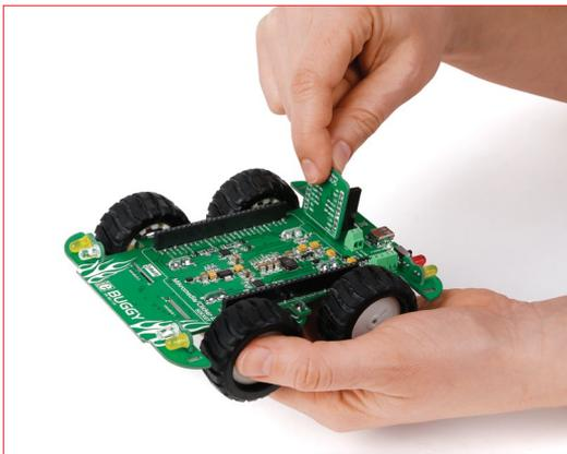
**STEP 7 -** Insert mikroBUS™ socket plates
