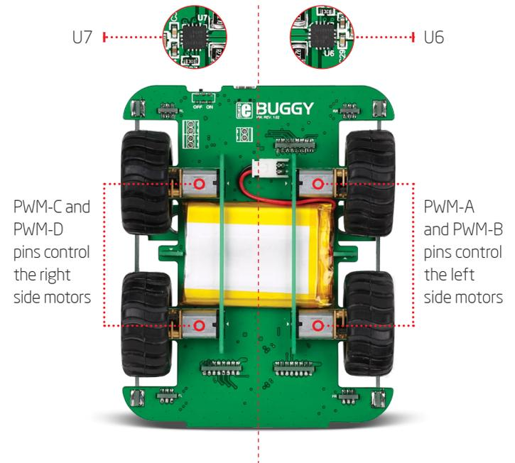
To prevent the motors from drawing too much current from the battery (and in doing so prevent the other components from functioning properly) a few resistors are placed to limit current draw. Each motor can draw a maximum of 400 mA, for a total of 1.6 A for all four motors.
